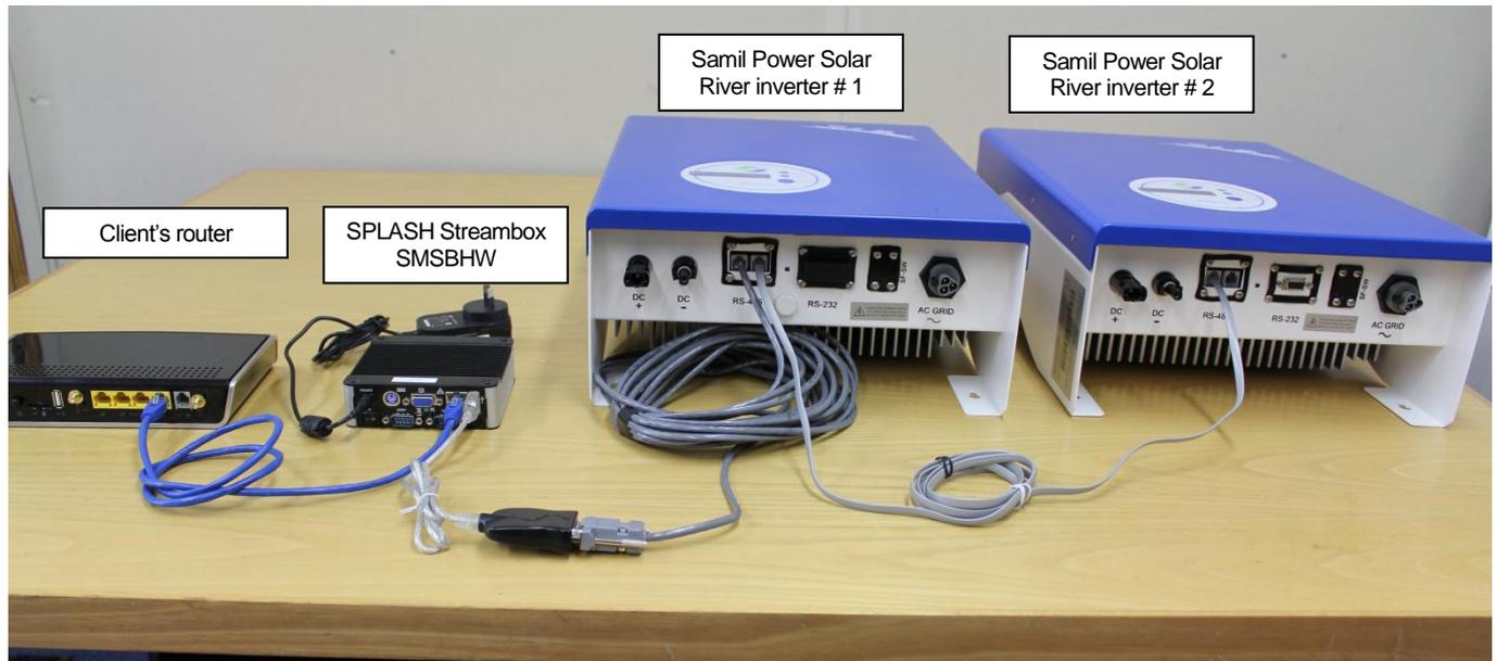
The photo above shows the connectivity between the various devices. The connections from left to right are:
